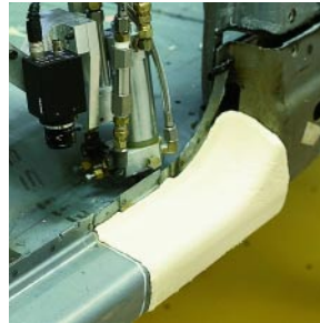
Left and center: BETAFOAM provides excellent cavity-blocking performance. Right: Air leak testing in Dow Automotive acoustical lab.
